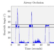
Figure 7. The thin blue line depicts airway occlusion during ventilations measured by the accelerometer; AHA guidelines recommend a head-tilt angle between 30 degrees and 35 degrees<sup>1</sup>.
