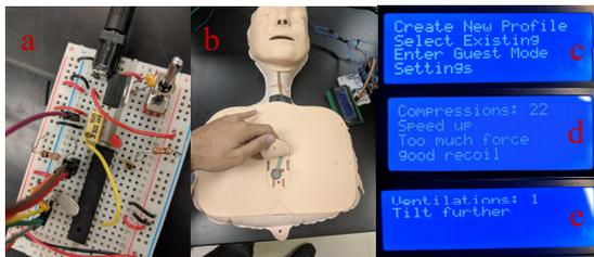
Figure 2 (a-c). Figure 2a displays a portion of the circuit; Figure 2b displays the force-sensitive resistor placement within the manikin; Figure 2c shows the initial options available to users; Figure 2d shows example feedback displayed on the LCD during compressions; Figure 2e shows an example of feedback displayed on the LCD during ventilations.
