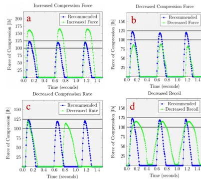
Figure 4(a-d). Data Generated from Manikin's Force Sensor. In each graph above, the blue line represents the recommended AHA guideline, while the gray lines represent upper and lower bounds for these metrics<sup>1</sup>. The green lines plot data from manikin sensors during training. Figure 4a displays excess compression force; Figure 4b displays insufficient compression force; Figure 4c displays insufficient compression rate; Figure 4d displays insufficient chest recoil.
